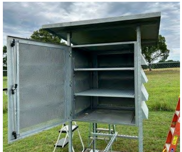
Figure 3. Collocation shelter with door open.
